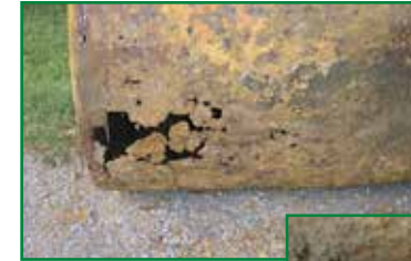
Ground contamination from a leaking underground tank
