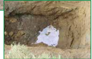
Ground contamination from a leaking underground tank
